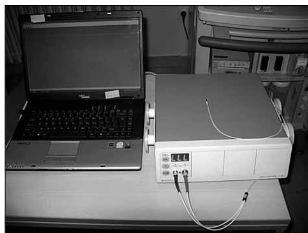
Figure 1. Laser Doppler device connected to the computer Slika 1. Laser dopler aparat povezan s računarom
