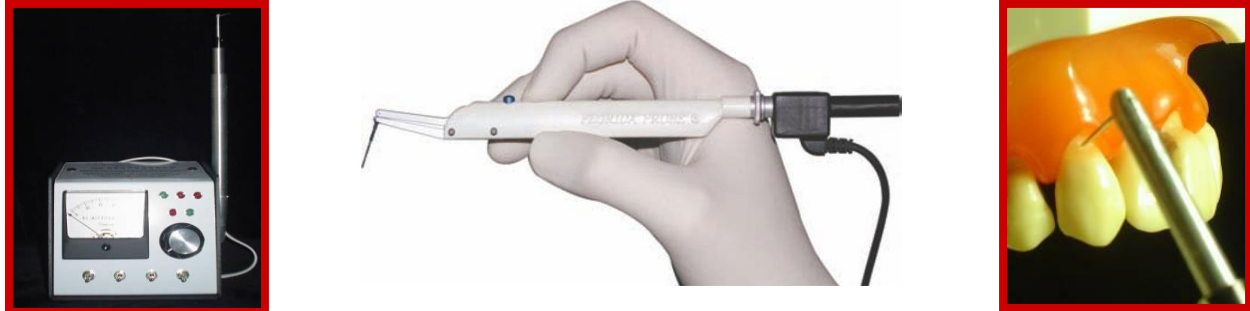
Slika 2. Electronic Force Sensing Probe (Yeaple sonda)
