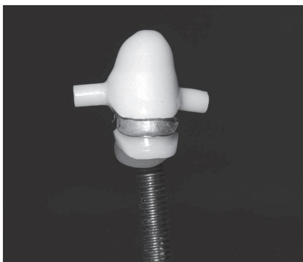
Figure 2. ZrO<sub>2</sub> secondary crown with electroplated gold coping
