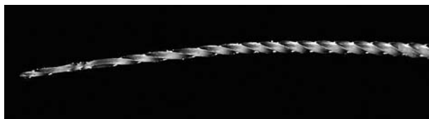
Figure 4. Deformation in a term of thread loss (K-file, 0.20) in the apical third of the working part after use on extracted teeth and sterilization in autoclave.
