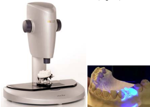
a) Cerec In Eos Blue 3D digitization system with the detail during the scanning process
