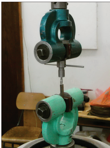
Figure 3. Detail of the universal testing machine just before the separation of metal cap from the abutment Slika 3. Detalj univerzalne servohidraulične kidalice neposredno pre odvajanja metalne kapice od nosača nadoknade
