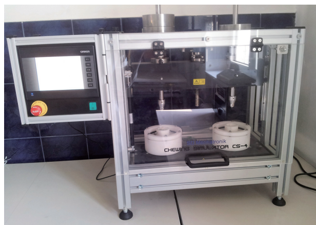
Fig. 6 Chewing simulator CS-4 (SD Mechatronik, Feldkirchen-Westerham, Germany).
